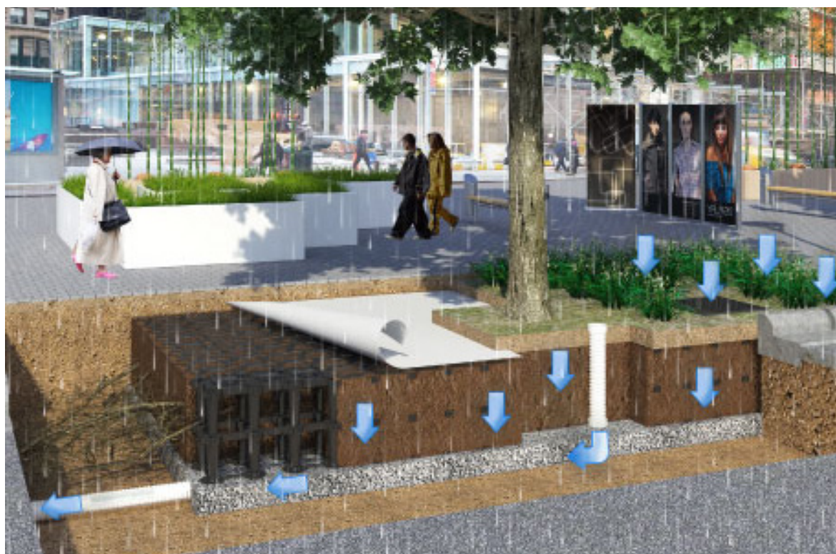
Figure 2. Strataflow™ Raingarden Stormwater Treatment/Storage System
