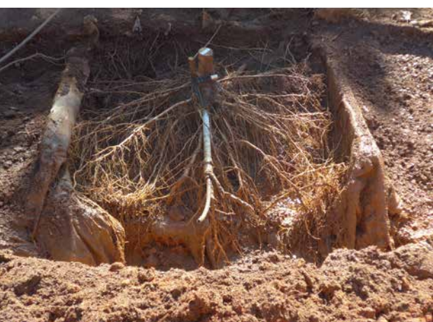
(Top) Fig 2.2.7 - Root distortion/restriction from structural soil (Middle.) Fig 2.2.8 - Gravel based structural soil. (Below) Fig 2.2.9 - Control tree.
