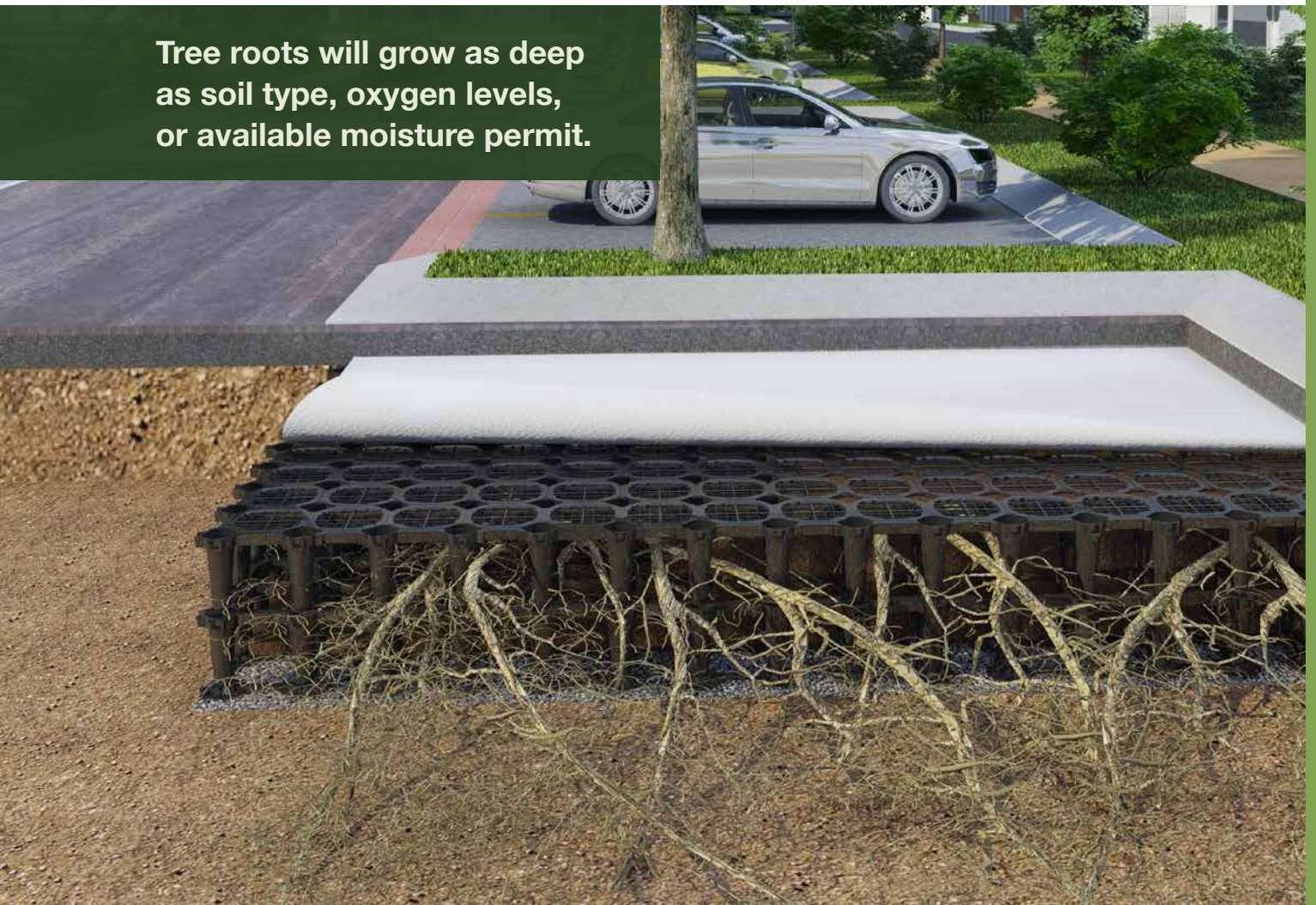
Fig 2.1.9 - High strength engineered soil cells permit large trees to be grown in road islands.
